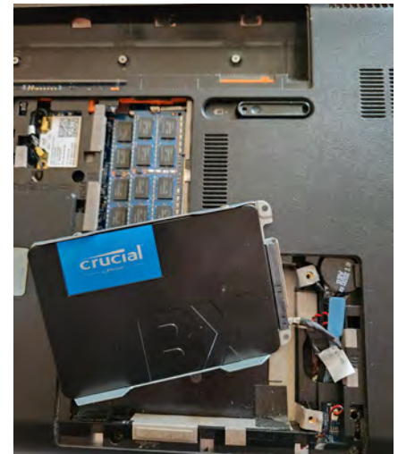
The HP Pavilion showing the SSD ready to be put back in the case.
